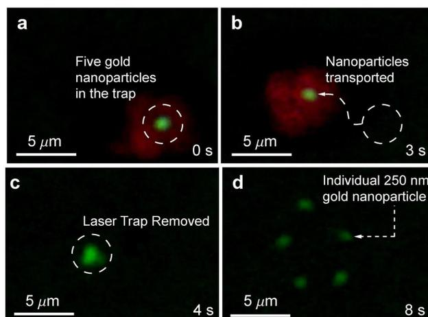
Figure 6: Trapping and transport of five 250 nm gold nanoparticles. (a) Nanoparticles are trapped and
