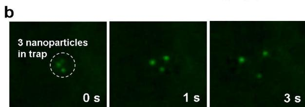
Figure 5: (a) The repulsive force ( $F_{rep}$ ) between two nanoparticles (due to dipole-dipole interaction and coulombic repulsion) as a function of applied voltage. (b) The repulsive force interaction is also observed for three nanoparticles. In the beginning, the particles are trapped using OET (laser filtered out), once the trap is removed, the nanoparticles repel each other.
