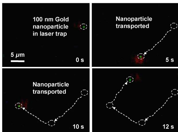
Figure 3: Trapping and transport process of a single 100 nm gold nanoparticle using OET. The nanoparticle is transported over an approximately 200  $\mu$ m<sup>2</sup> area in 12 seconds.
