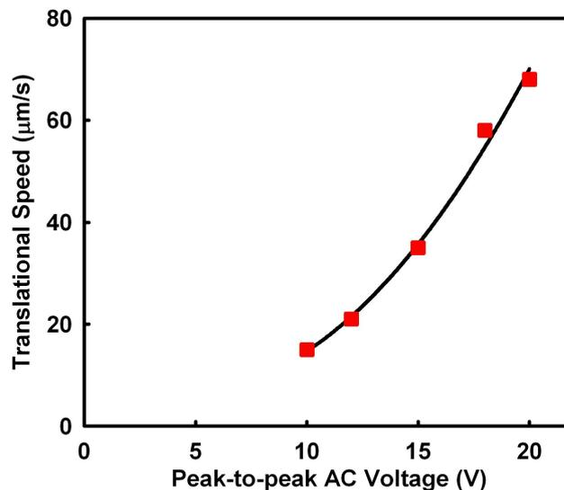
Figure 4: OET-trapped nanoparticles' translational speed as a function of the applied voltage. A maximum translational speed of 68  $\mu$ m/s at 20 Vpp is achieved. The experimental data follows a quadratic trend (black fitted curve). This is expected since the DEP force is proportional to  $\nabla E^2$ .
