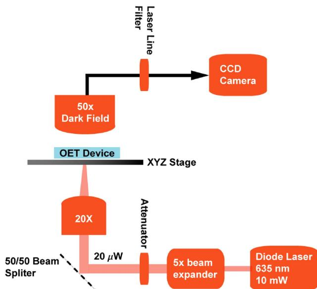
Figure 2: Experimental setup for manipulation of metallic nanoparticles. A 10-mW, 635 nm diode laser was expanded 5 $\times$ , attenuated to 20  $\mu$ W, and focused onto the OET chip with 1.7  $\mu$ m (FWHM) using a 20 $\times$  objective lens. The nanoparticles were visualized using dark field microscopy and a CCD camera.
